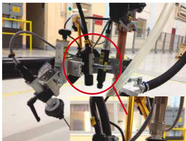
Camera installed onto bracket for welding torch
