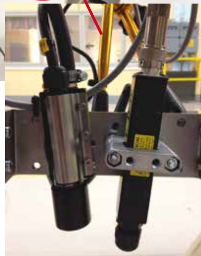
Camera installed onto bracket for welding torch
