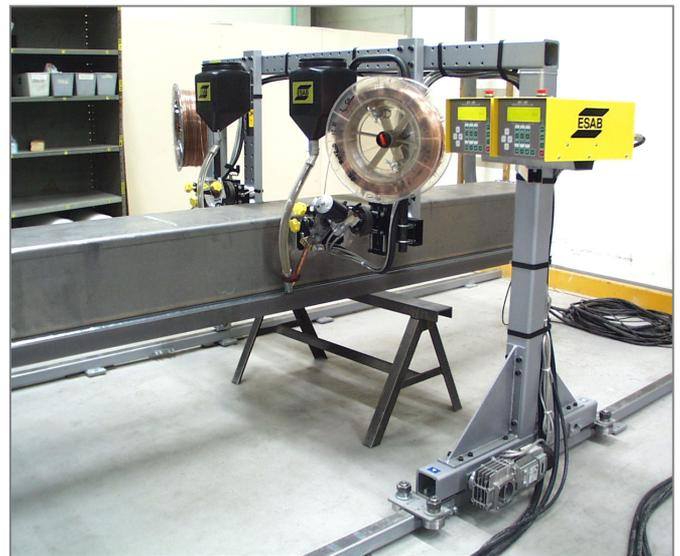
When MechTrac is equipped with driving motor on both sides, one will be master motor and the other one slave motor. The single or master motor is equipped with tacho. The gantry can support a maximum weight of 220 kg, which corresponds to two A2 welding heads, single or twin wire, complete with automatic joint tracking GMD and the OPC flux recovery unit, for example.
