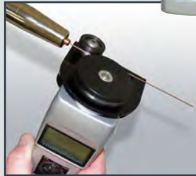
HHSS-12 obtaining measurement at the torch end
